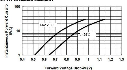
Fig.3-Typical Instantaneous Forward Voltage Characteristics
